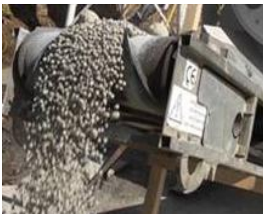
Figure 10: Pellets leaving process conveyor
